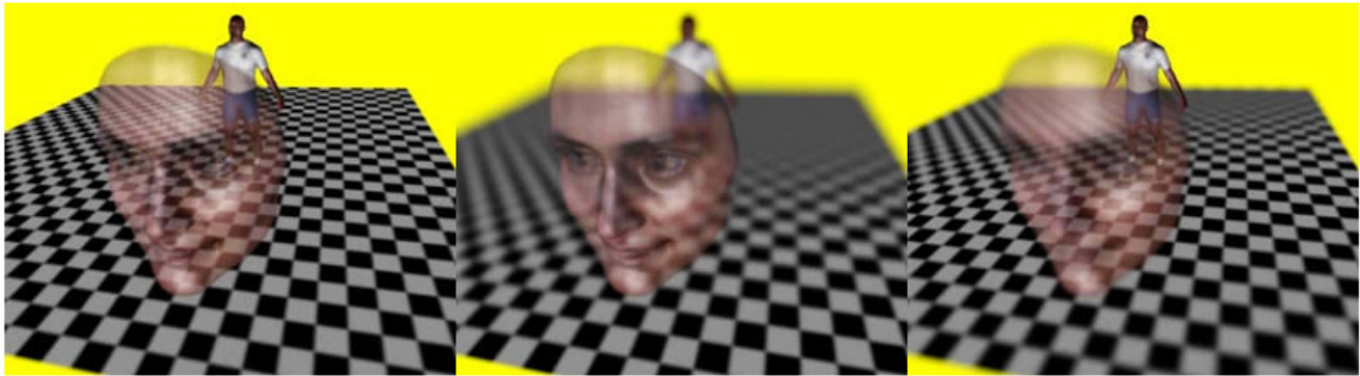
Figure 5: Example of ODF rendering with semitransparent surfaces. Left: no DOF. Middle: DOF is on and transparent mask is in focus. Right: the male body is in focus, the mask is out of focus.[7]
